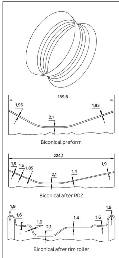
To produce even lighter steel wheels, machines have been developed which partially thin-out, and thus also widen, the blank (bandage) upstream of the rim roller. This permits production of steel wheels lighter by up to 25%.
