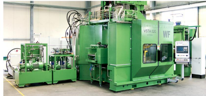
**Machine is part of the vertical ring Flow forming Center (RDZ).**
